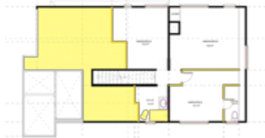
Demolition plan - Second floor
