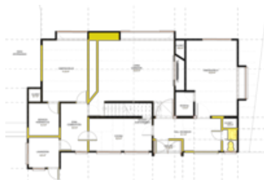
Demolition plan - First floor
